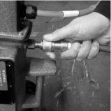
5. Connect your 50FT power cord to the twist lock pigtail on the heater (#4 on page 8). Plug the 50ft power cord(s) to the twist lock pigtail on the back of the machine (#6 on pages 6&7)
