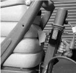
3. Connect your heater's inlet hose (#1 on page 8) to the machine's outlet quick disconnect (#7 on pages 6&7).
