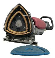
Thanks to the innovative Delta Cleaning System with orbital drive, the operator can determine the working speed at any time and thus precisely approach narrow areas and corners. The flat cleaning head is designed in such a way that cleaning close to walls, deep into corners and under furniture and substructures with an underclearance of as little as 4.72" is possible.
