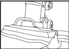
**Install the Dust skirt, align the dust skirt velcro, with the Velcro strips you installed on the chassis.**
