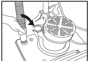
6.- Connect the hose to the machine coupling and insert the hose into the hose clamp. It's possible to connect 1 1/2" or 1 3/4" diameter hoses.
