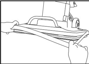
1.-Remove the yellow bumper guard by pulling it off the chassis.
