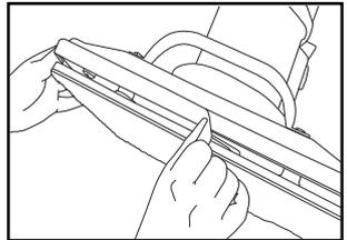
3.-Remove the paper backing from the Velcro strip and following the base edges apply around the machine. Make sure to press the velcro firmly against the base for maximum adherence.
