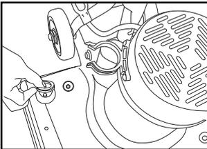
5.- Install the hose clamp on the motor cover. Use the 2 screws included in this kit. And remove the cap off the hose coupling.
