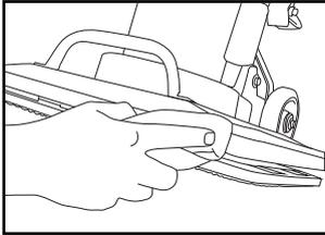
2.-Clean the edges of the chassis with a clean wipe, use a degreaser or alcohol to remove debris and grease.
