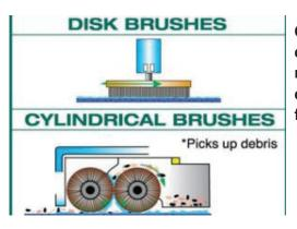
Cylindrical scrubbing utilizes counter rotational brushes that mechanically lift debris while cleaning. Brushes turn in opposite direction of each other and facilitate pre sweeping for many applications. It is especially effective for all types of three dimensional flooring with it's unique ability to clean deeper in uneven surfaces.
