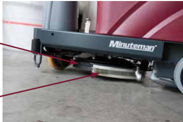
Wide 26" Auto load & Unload pad driver or brush
