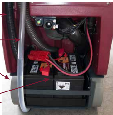
Easy Access to Batteries
